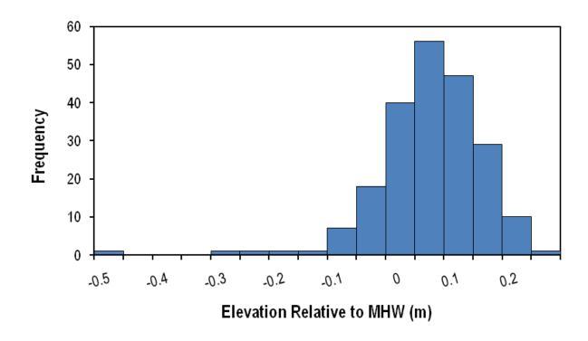
Figure B-2. Distribution of elevation samples relative to local mean high water (MHW) at Black John.
