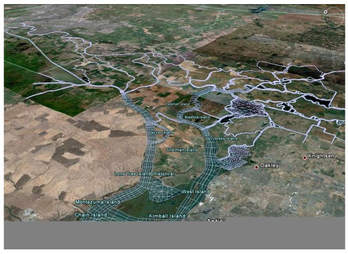
Figure 26. Example of the Unstruc grid in the Delta. The irregular polygon shapes allow computationally efficient modeling of complex geometries.
