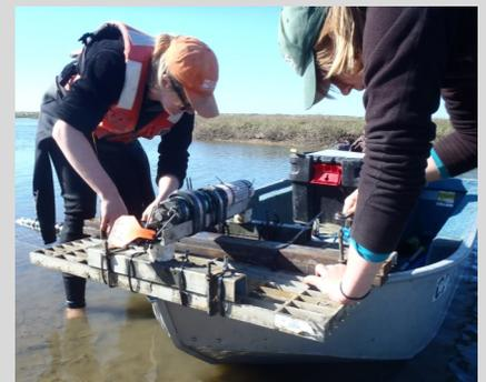
Technicians deploying a current profiler to better understand site specific sediment dynamics.
