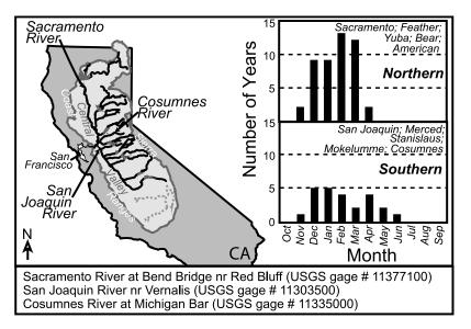
**Figure 1.** Sacramento-San Joaquin River system watershed; arrows point to location of three gaging stations. Bar charts show distribution of levee breaks indicating number of years with breaks occurring during particular months of the year for northern and southern portion of the system.
